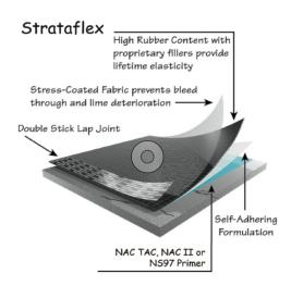
Strataflex\* substantially reduces reflective cracking and delamination between the substrate and floor surface and because it is a self-bonding system, it is easier to apply, and installs faster than other systems. Once applied, floor tile can be installed immediately, minimizing down time and labor cost.
